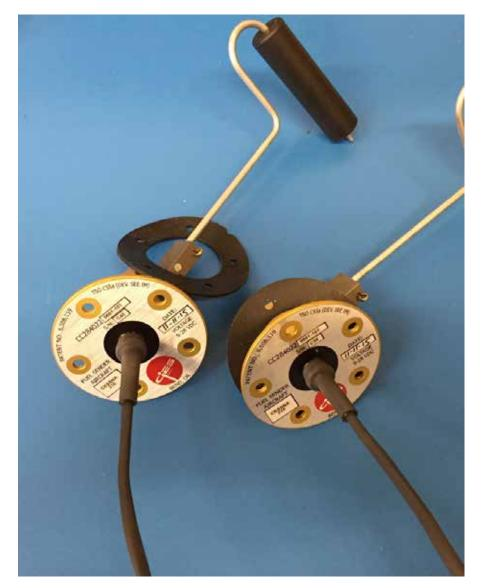
but it uses magnetic field technology instead of the old resistive system. The change in the magnetic field is transmitted to a digital cockpit gauge, which registers the fuel level to degrees of accuracy not thought possible in a fuel gauge.
