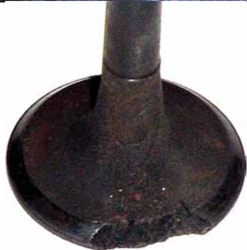
Figure 1—This exhaust valve failed in-flight, shutting down the cylinder.
