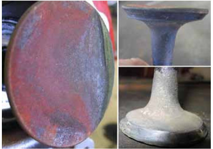
Figure 3—A badly burned exhaust valve. Note the hot spot (left panel, 2-4 o'clock), the warping (top-right panel), and metal erosion (bottom-right panel). This valve was only hours from complete failure.
