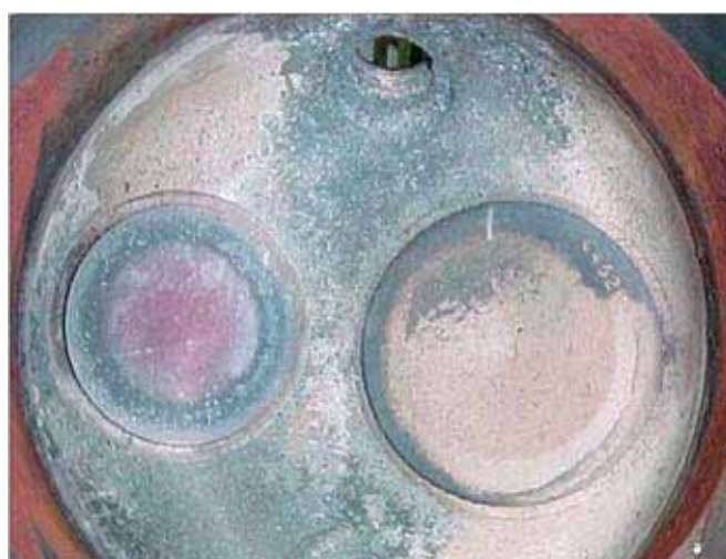
Figure 5—Note the symmetrical appearance of the exhaust valve (left), showing the valve is operating normally
