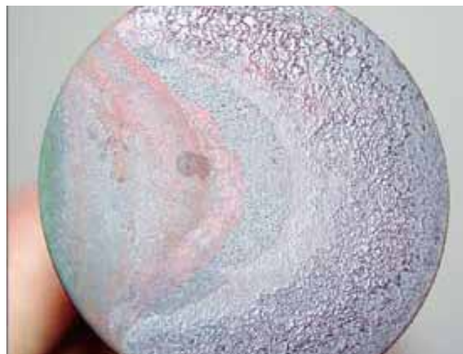
Figure 6—This exhaust valve is in serious trouble, and doesn't have much longer to live. There's an obvious hot spot in the 8 to 10 o'clock position.
