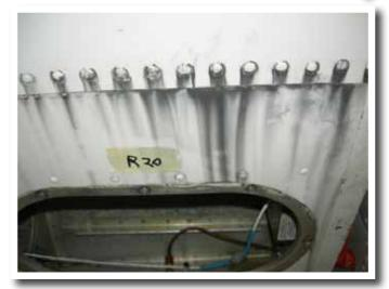
The wing spar rivets need replacement at the SID inspection if they are working loose. The Americans call them "smoking rivets".
