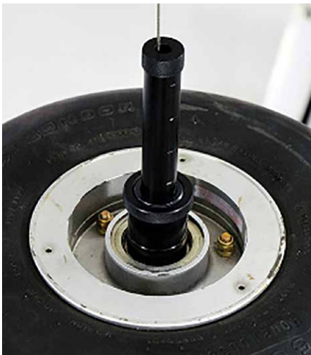
Example of Static Wheel Balancing
