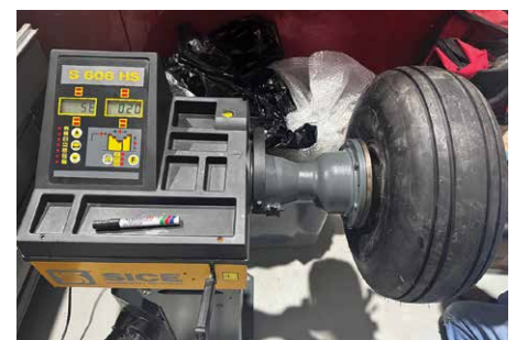
Example of Dynamic Wheel Balancing
