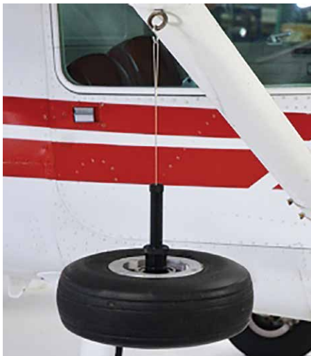
Example of Static Wheel Balancing
